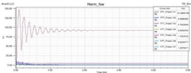
Figure 5: Expected amplitudes of the harmonics of the coil current at an operating frequency that is below the resonant frequency of the system (below resonant operation)
