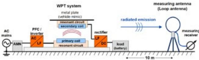
Figure 8: Principle measuring the magnetic field strength with a loop antenna for evaluation of the emitted EMC interference in the frequency range between 9 kHz and 30 MHz
