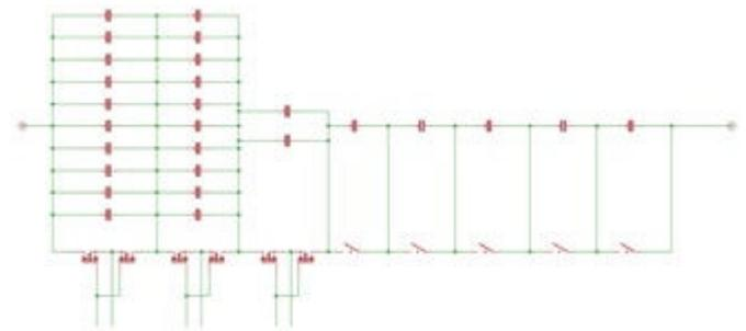
Figure 1: Circuit for variable tuning of an inductive charging system as implemented in the research project
