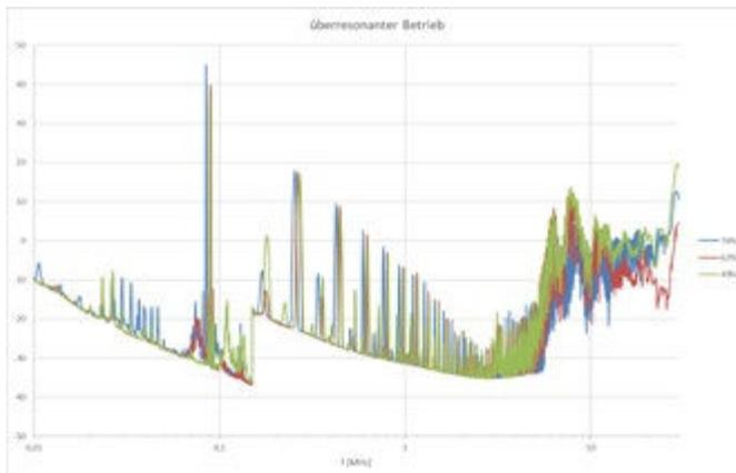
Figure 9: Magnetic field spectrum during operation with different tunings of the resonant circuit, out of resonance in each case
