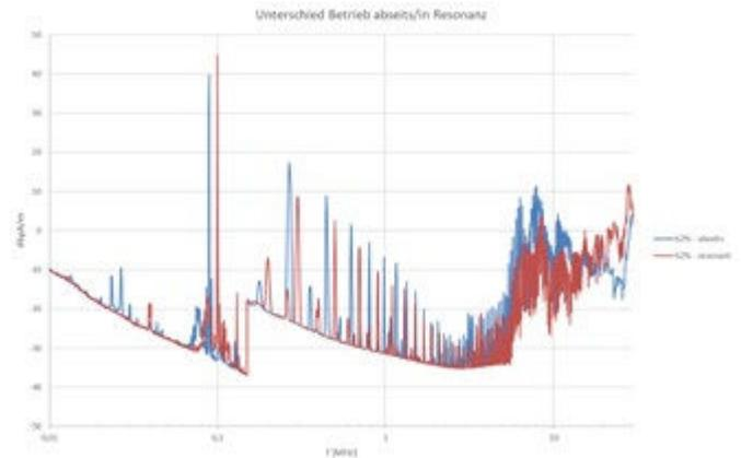
Figure 11: Magnetic field spectrum during operation with the same resonant circuit tuning (but different to Figure 10), with different frequencies (out of/in resonant mode)
