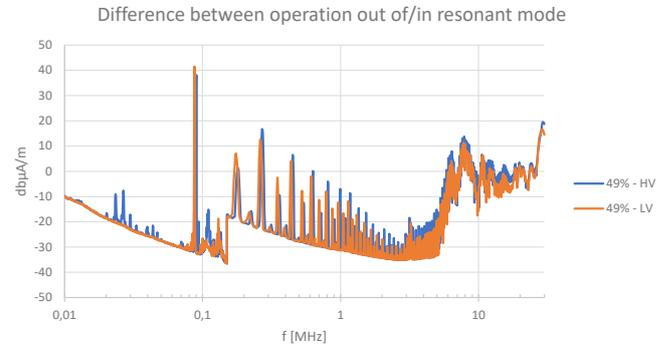
Figure 10: Magnetic field spectrum during operation with the same resonant circuit tuning, with different frequencies (out of/in resonant mode)
