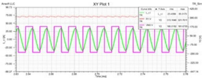
Figure 2: Expected current and voltage forms at the transmitter coils at an operating frequency that is above the resonant frequency of the system (above resonant operation)
