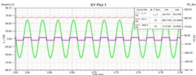
Figure 6: Expected current and voltage forms at the transmitter coils at an operating frequency that corresponds to the resonant frequency of the system (resonant operation)
