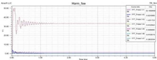
Figure 3: Expected amplitudes of the harmonics of the coil current at an operating frequency that is above the resonant frequency of the system (above resonant operation)
