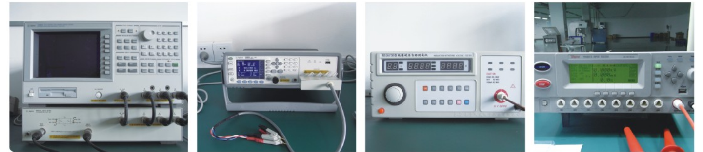
网络/频谱/阻抗分析仪Network/Spectrum/ Impedance Analyzer (Agilent 4395A) 精密LCR测试仪Precision LCR Meter (Agilent E4890A) 绝缘耐压自动测试仪 Insulation Withstand Voltage Tester 耐压测试仪Hipot Tester
