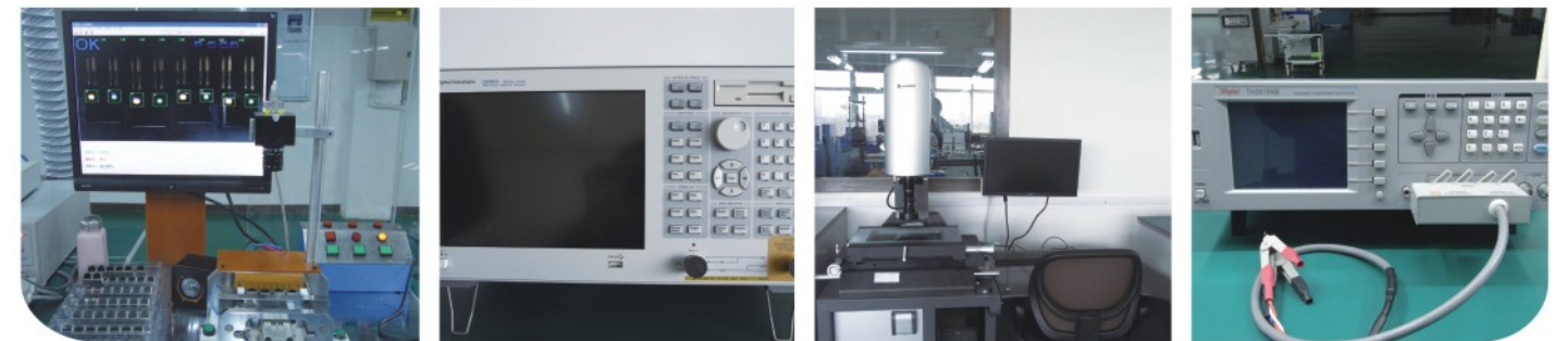
LED自动测试仪LED Automatic Test System 网络分析仪ENA Series Network Analyzer (Agilent E5061A) 二次元测试仪 Quadratic Element Tester 变压器综合测试仪 Automatic Transformer Test System
