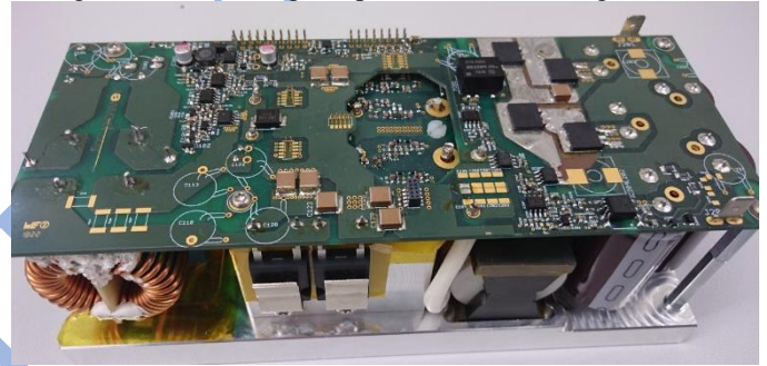
Figure 3 - Final demonstrator of Single-stage OBC in open-frame configuration
